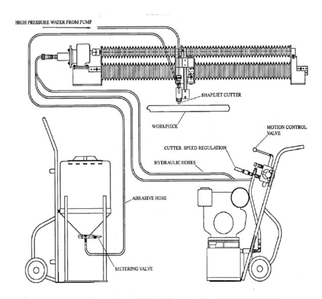
ABRASIVE HOPPER WITH METERING VALVE
